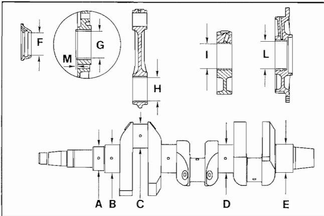
**Main bearing and connecting rod big end bearing inside diameter**
