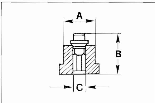
**Injection pump delivery valve (same for all engines of the series)**
