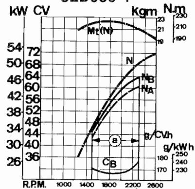
**N (DIN 70020) AUTOMOTIVE RATING:** intermittent operation with variable speed and variable load.
