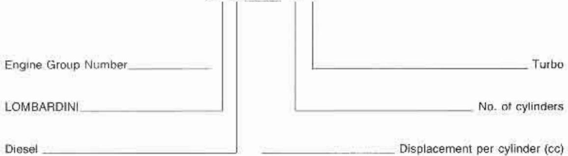
Once you have identified the model number you can identify the engine by means of the Ser. No. indicated on the name-plate applied to the blower stator and the crankcase.
